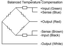
The two "sense" wires sample the bridge supply voltage at the load cell. Complete compensation of change in the lead wire resistance, due to temperature change and / or cable extension, is achieved by feeding this voltage into appropriate electronics.
